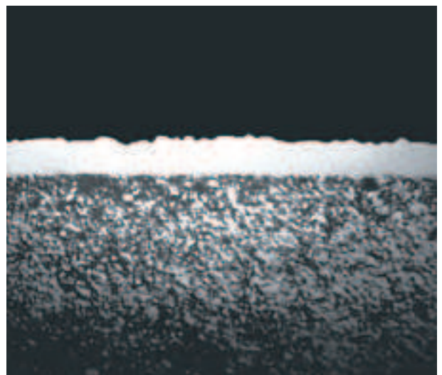
Fig. 8.2: Cross section of the ATCoat coating
